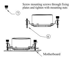
Screw mounting screws into motherboard and tighten with mounting nuts
