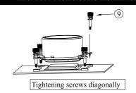
Align holes of fixing plate and lock with fixing plate screws
