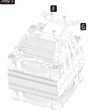
Place INTEL bracket on the cooler base, and then use bracket
