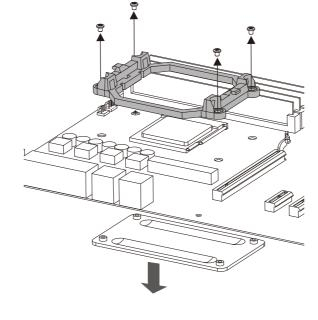
Please remove the original heatsink mount holder before further installation.
