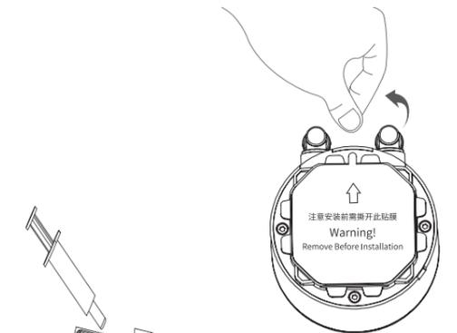
Applying thermal paste on CPU/ Remove the protection film
