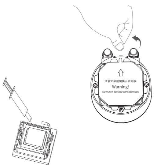
Applying thermal paste on CPU/ Remove the protection film
