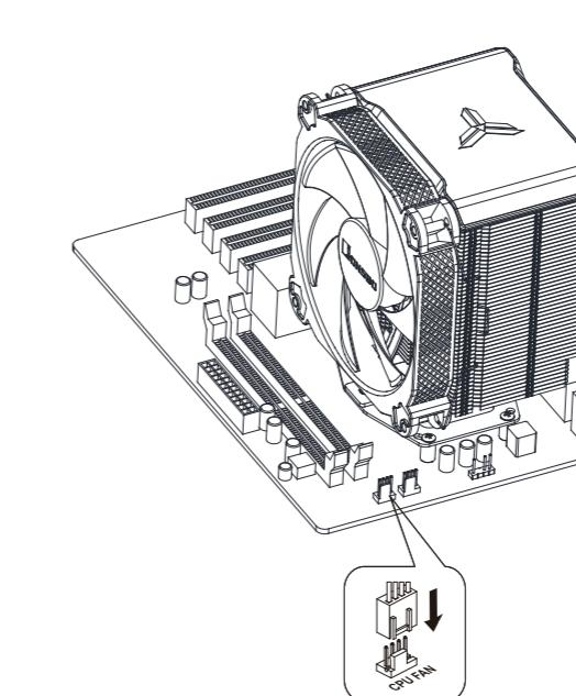
Connect fan cables to CPU\_FAN socket
