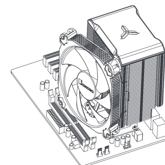
Insert the top cover back on cooler, secure the fan with fan clips
