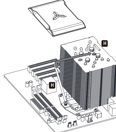
Place the cooler on the CPU, remove the magnetic top cover, and secure the base screw to the mounting bracket.
