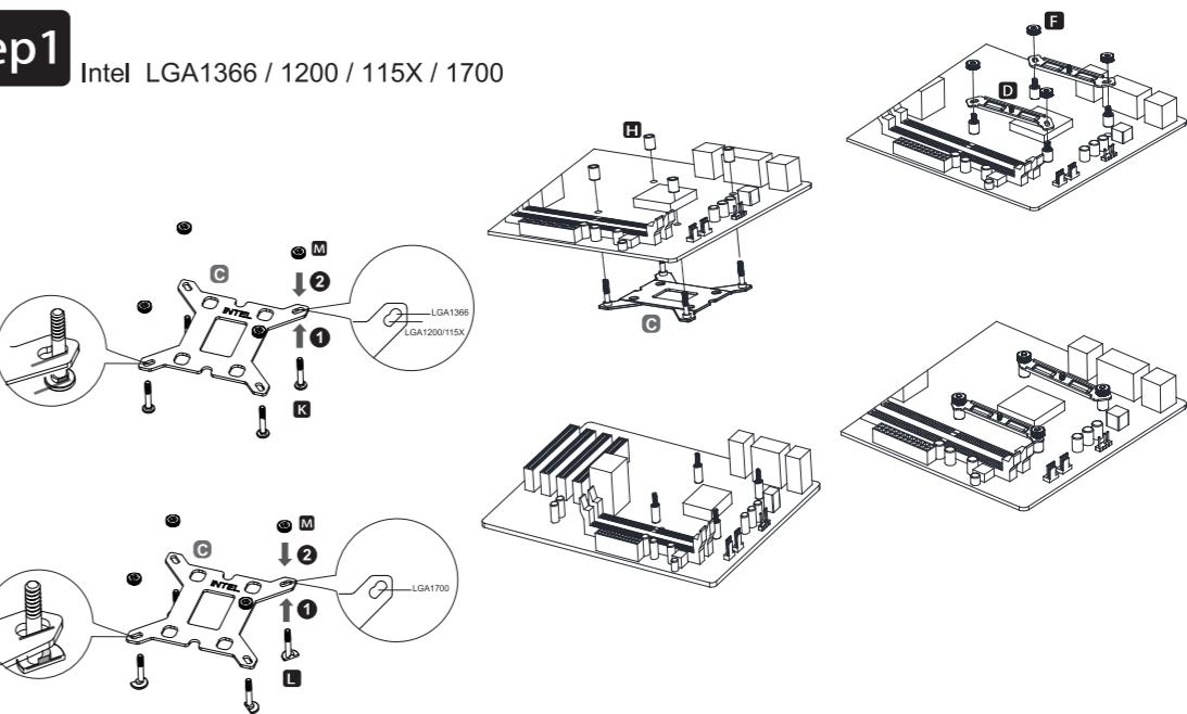
Install the backplate to the motherboard and fix it with spacers
