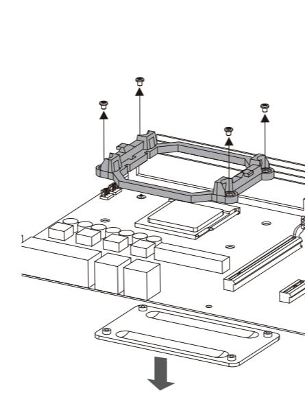
Remove the plastic retainer of the AMD retention module, place the existing backplate back to MB
