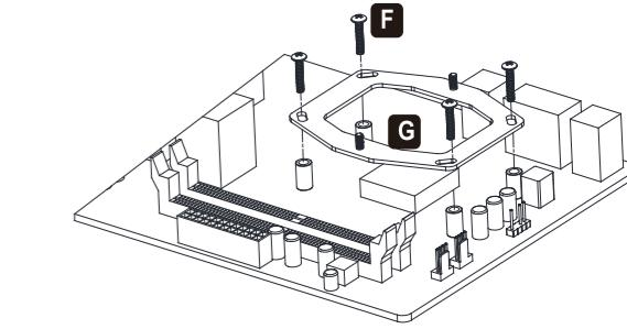
Install the AMD mounting plate and secure with position screw
