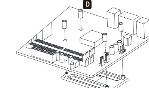
Install the spacer to secure the AMD backplate
