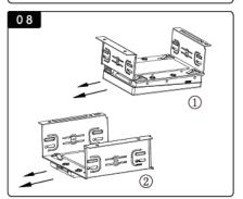
光驱架底部为第二硬盘位, 图①为3.5寸硬盘的装入方式, 图②为2.5寸硬盘的装入方式。 箭头方向为数据接口方向。 The second hard disk should be installed on the bottom of CD-Rom bracket and the connector of hard disk should face the pointing directions. For installing 3.5 inch hard disk, please refer to diagram ①; for installing 2.5 inch hard disk, please refer to diagram
