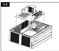
放入主板,用螺丝锁固。 Install the motherboard, and then screw and lock it.
