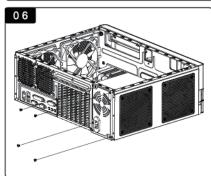
放入电源,用螺丝锁固。 Install the power supply, and then screw and lock it.
