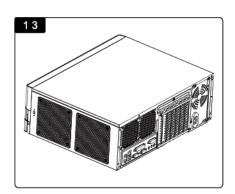
装回顶盖并以螺丝锁固。 Install the top cover, screw and lock it.
