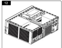
装入硬盘架,连接数据线。 Install hard disk bracket, and then connect all the cables.
