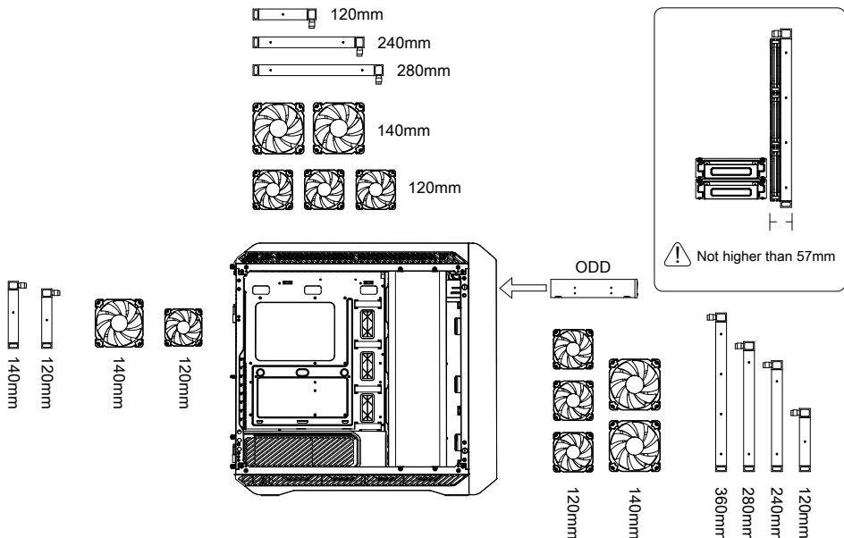
\*When the 3.5" HDD installed in the inner compartment of the case (horizontal hard drive rack), the total thickness of the 360/420 radiator support at the front of the case is 57mm
