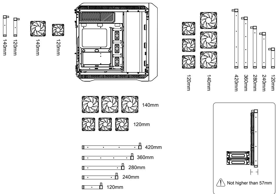
\*The installation position of the 420 radiator could be install at the front or on the bottom cover, and the maximum radiators size and amount is 420mm\*1 + 360mm\*1
