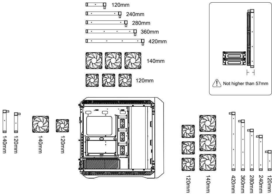
\*The installation position of the 420 radiator could be install at the front or under the top cover, and the maximum radiators size and amount is 420mm\*1 + 360mm\*1
