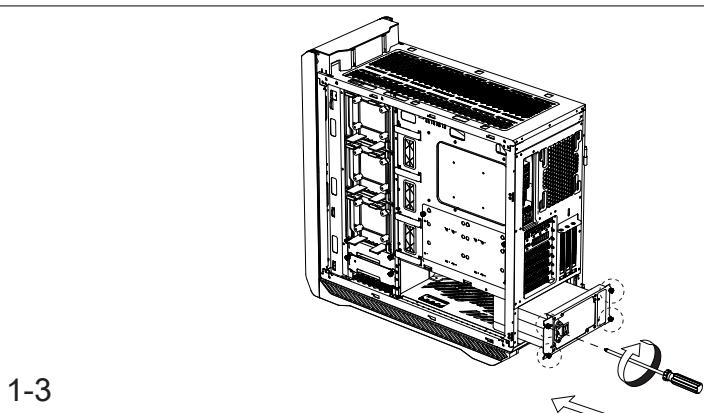
Horizontal GPU mounting installation steps
