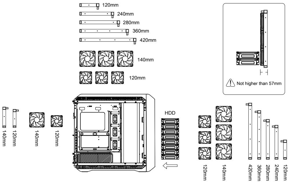
\*The installation position of the 420 radiator could be install at the front or under the top cover, and the maximum radiators size and amount is 420mm\*1 + 360mm\*1
