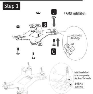
When using the AMD CPU ,Please let the words AMD on the upside. Fix the locating screw on the corresponding hole according to the requirement of the main board.
