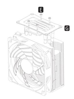
Install the bracket mount on the cooler base. Fasten the bracket mount
