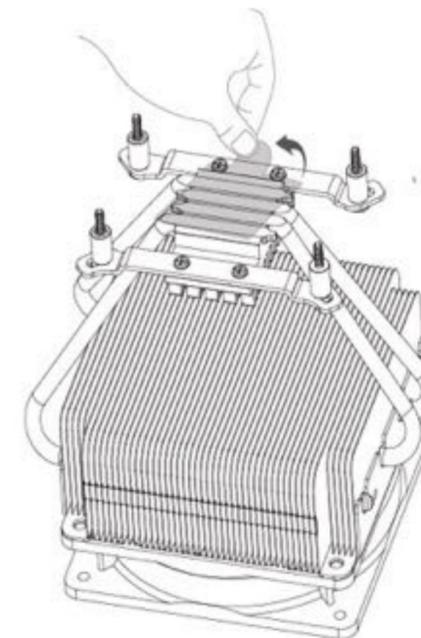
**EN** Remove protective film before installing the cooler.
