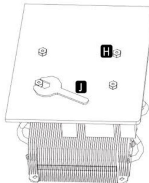
**EN** Fix the coolers on the motherboard by fixing the hex nuts with the wrench.
