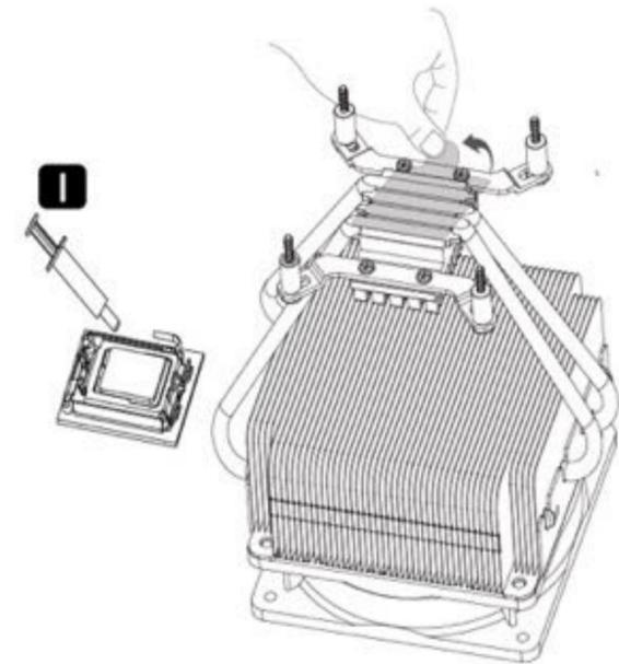
**EN** Evenly apply the thermal grease onto the CPU, and remove the protective film from the cooler base.
