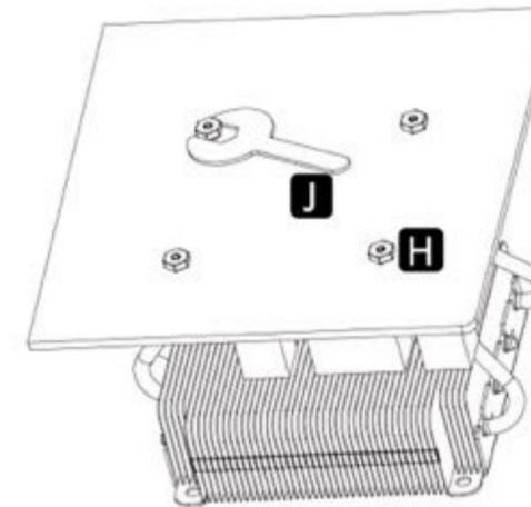
**EN** Fix the coolers on the motherboard by fixing the hex nuts with the wrench.
