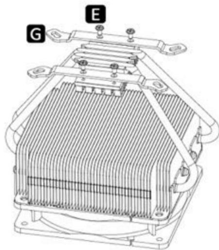
**EN** Install AMD bracket on the cooler base, and then use bracket screws to fix it.
