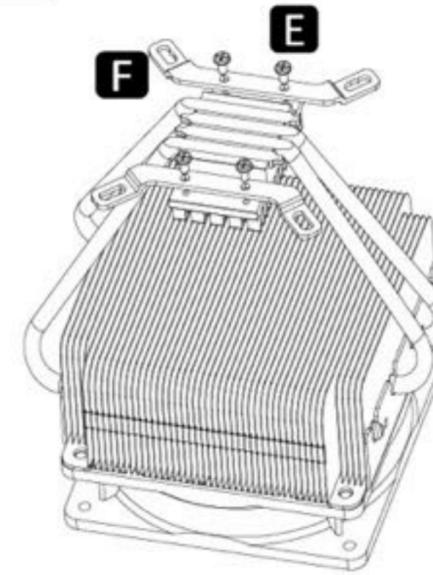
**EN** Place INTEL bracket on the cooler base, and then use bracket screws to fix it.
