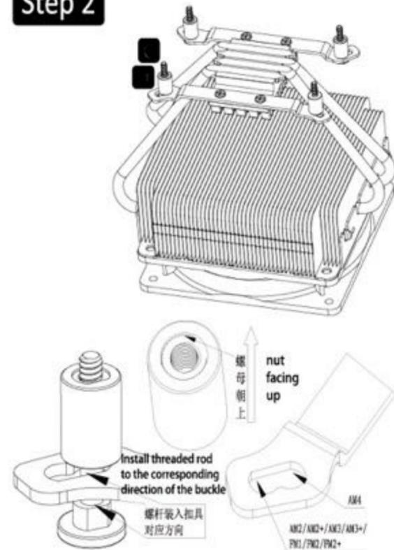
**EN** Install threaded rod to the corresponding holes of AMD bracket as needed, fixing it with nut facing up.
