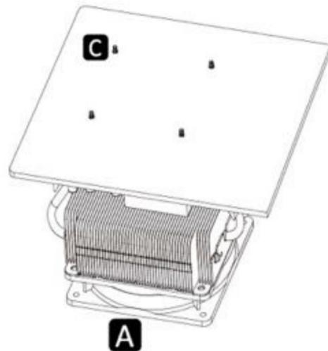
**EN** Pointing the holes of the motherboard to the positioning screws of the cooler, and then assemble them together.
