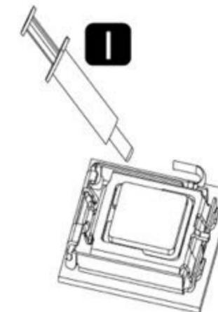
**EN** Evenly apply the thermal grease onto the CPU.
