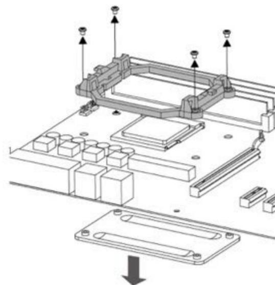
**EN** Please remove the original heatsink mount holder before further installation.
