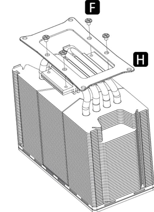
**EN** Install the bracket mount on the cooler base. Fasten the bracket mount with screws.
