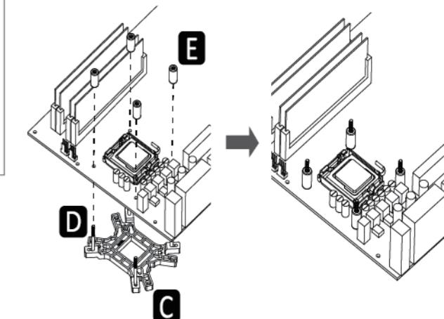
**EN** Insert the position screws into the proper holes on the back plate.
