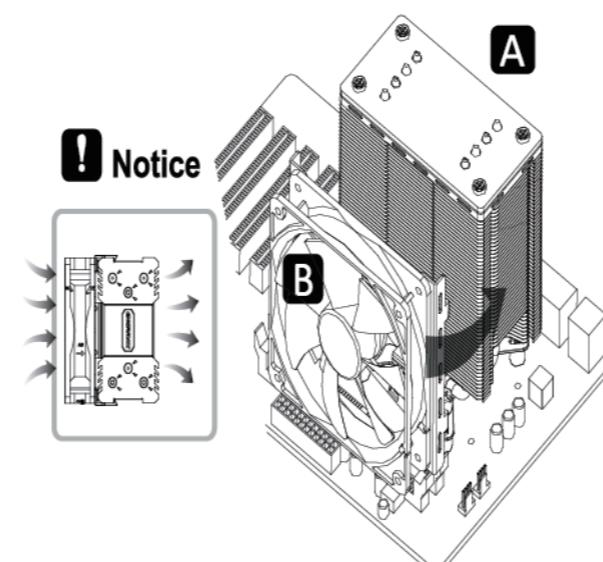
**EN** Attach the fan to the cooler with fan brackets.
