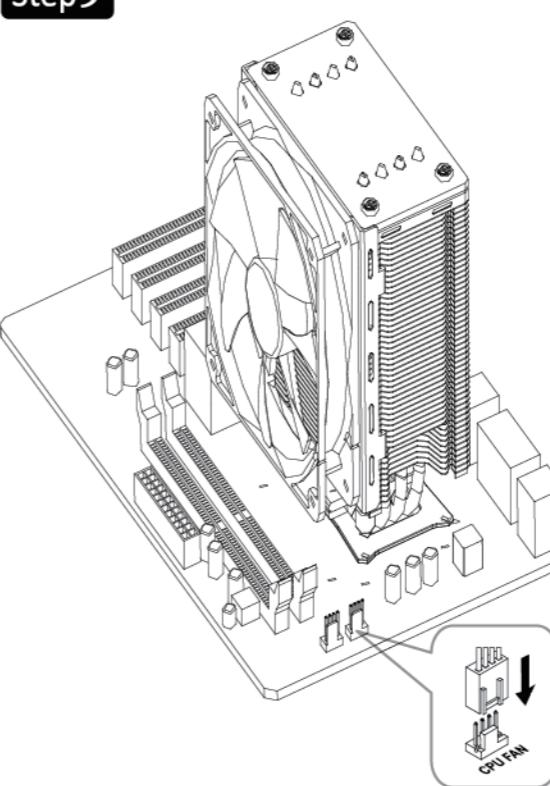
**EN** Connect the fan 4 pin header to the CPU fan power socket on the motherboard.
