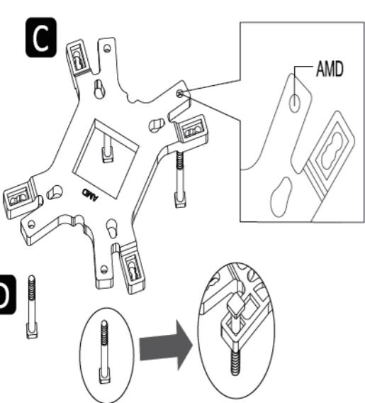
**EN** Insert the position screws into the AMD holes on the back plate.
