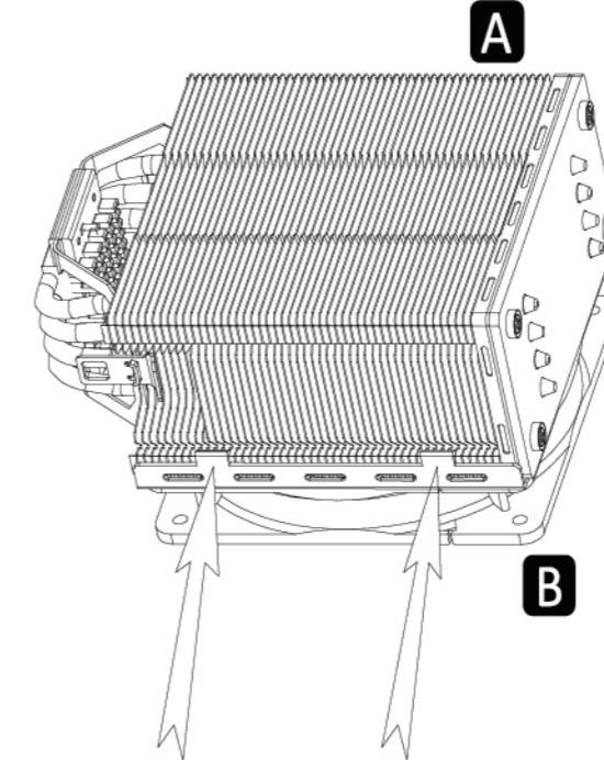
**EN** Please remove the fan before installing radiator by opening those 2 buckles pointed by arrow.
