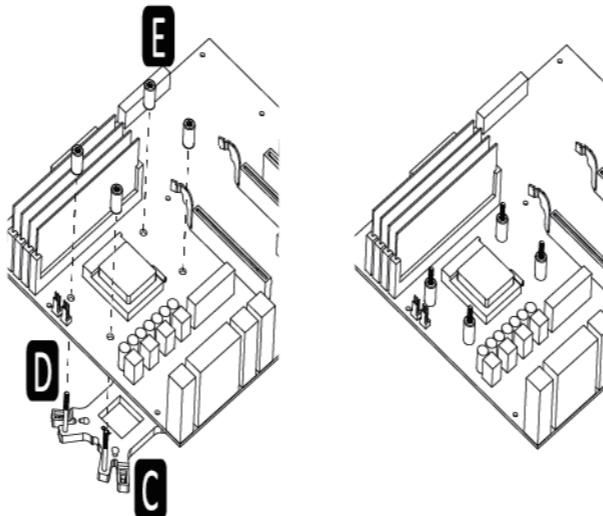
**EN** Install the back plate on to the back of the motherboard. Put the stand-offs into the back plate screws.
