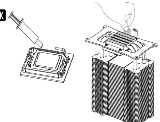
**EN** Apply the thermal grease evenly onto the CPU surface.
