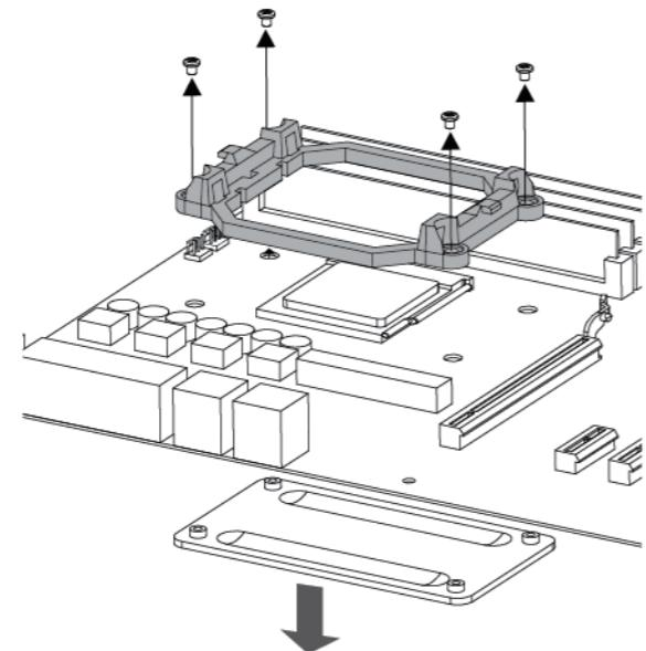
**EN** Please remove the original heatsink mount holder before further installation.
