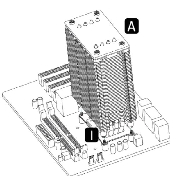
**EN** Place the cooler on the CPU and tighten the fixed screws until all four corners are secured.
