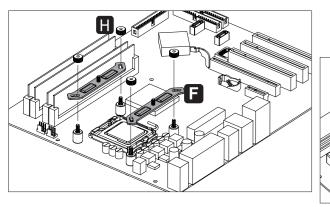
EN Install the mounting plates on the position screws and fasten the nuts
