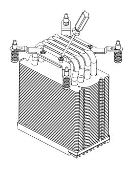
Please remove the fan before installing radiator by opening those 2 buckles
