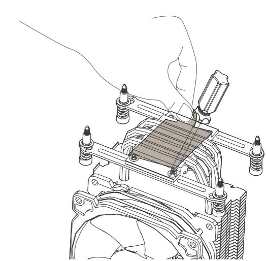
Install the AMD brackets to the fixing point of the cooler with screws, and then remove the protective film
