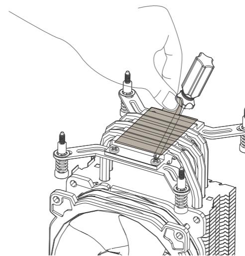
Install the Intel brackets to the fixing point of the cooler with screws, and then remove the protective film
