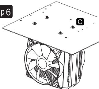
**EN** Pointing the holes of the motherboard to the positioning screws of the cooler, and then assemble them together, install insulating washers
