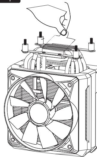
**EN** Please remove the protective film before installing the cooler
