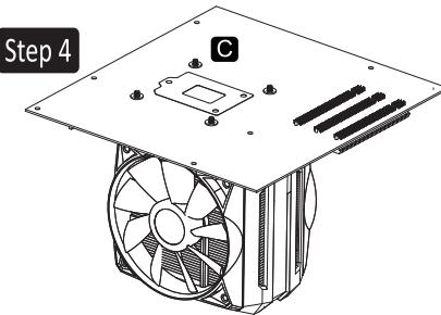
EN Pointing the holes of the motherboard to the positioning screws of the cooler, and then assemble them together, install insulating washers
