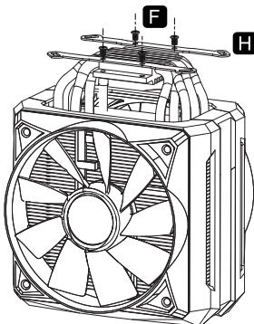
**EN** Install AMD bracket on the cooler base, and then use bracket screws to fix it
