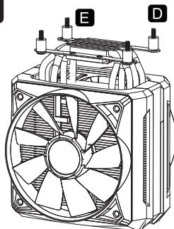
Install threaded rod to the corresponding holes of AMD bracket as needed,fixing it with nut facing up
