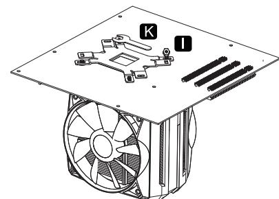
EN Fix the coolers on the motherboard by fixing the hex nuts with the wrench
