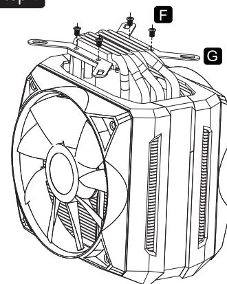
EN Place INTEL bracket on the cooler base, and then use bracket screws to fix it
