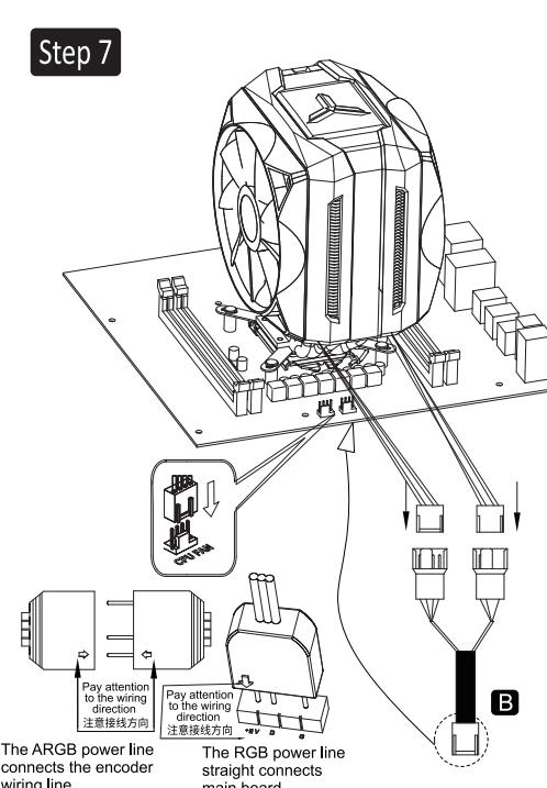
EN Use Y cable to connect the two fans of the coolers (as shown in the figure), then connect Y Cable to the motherboard. At the same time, connect the 5V ARGB lamp line to the host or connect it to the encoder wiring as required
