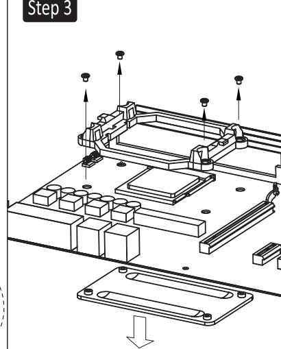
**EN** Please remove the original heatsink mount holder further installation
