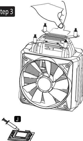
EN Apply the thermal grease evenly on to the CPU surface.
