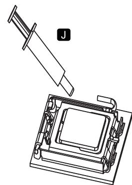
**EN** evenly apply the thermal grease evenly on to the CPU surface
