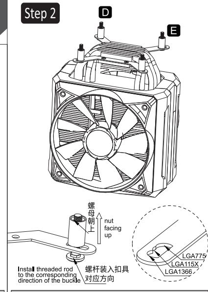
EN Install threaded rod to the corresponding holes of INTEL bracket as needed, fixing it with nut facing up
