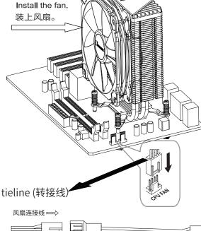
Place the radiator on the CPU while aligning the support screw to the backplane nut and tightening (Pictured above)
